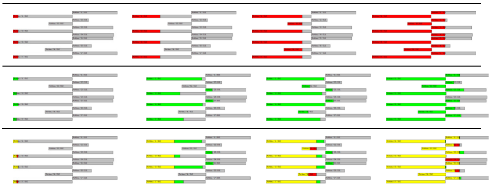
Fig. 6: colored Gantt chart at five points in time of the progress reports: target values (top), actual values (center), overlay (bottom)
