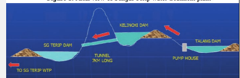
Figure 2: Schematic view of water storage
