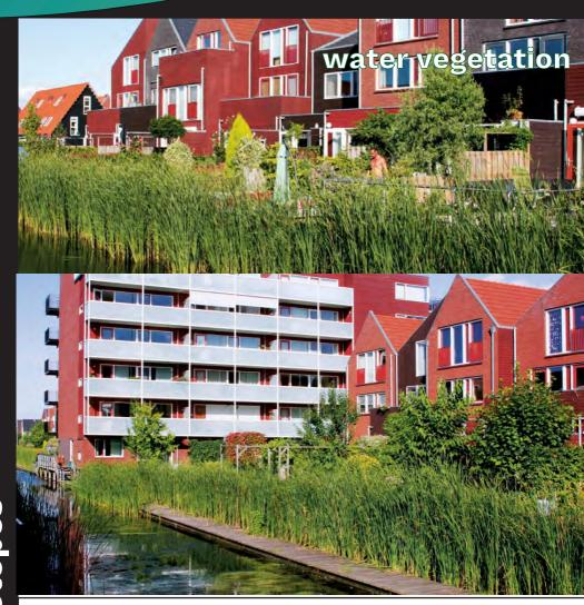
Green riparian zones form a gradual transition from shore to the water. It has a positive impact on water quality. Reeds and rushes absorb nutrients, and floating particles settle on them, as a result of which the clarity of the water improves.
