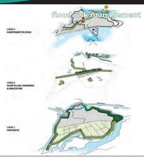
Dividing a large dike ring into a number of smaller compartments, even within urban areas, can limit the consequences of flooding to a smaller area.
