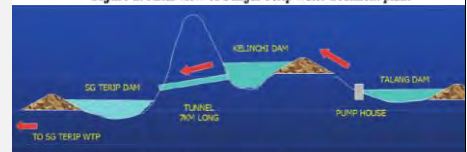
Figure 2: Schematic view of water storage
